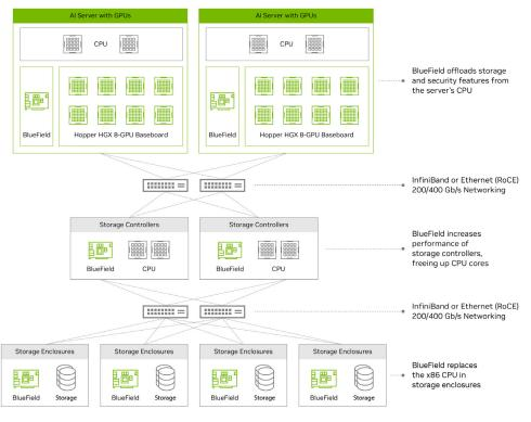
BlueField enhances storage performance, security, and efficiency in the server, storage controller, and storage enclosure.
